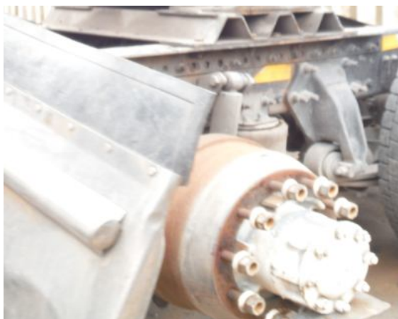
Axle 2 left – tyres missing
